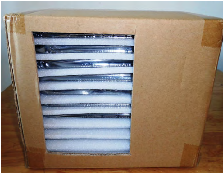
Place Foam Sheets and Trays into Box
